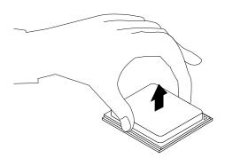
Figure 34. Removing the microprocessor
